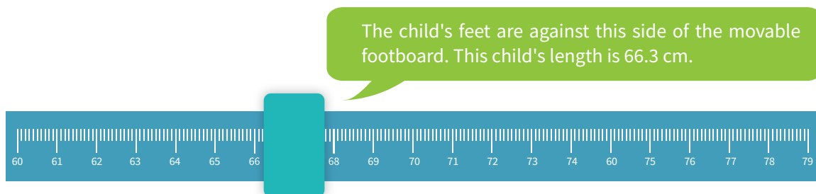
Figure 14. Example for reading measuring tape
