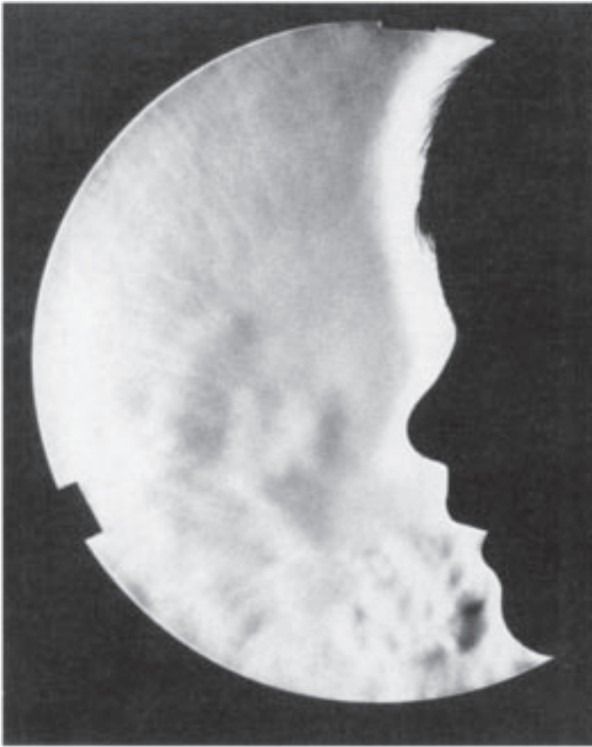
Figure 6.13 Schlieren photograph of a child's face showing regions of relatively warm air (light) and cool air (dark). The light layer immediately adjacent to the face is the laminar boundary layer (after Gates, 1972).
