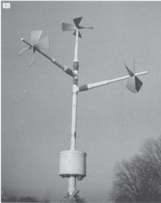
Figure A2.3 (a) Cup anemometers (right) installed to measure the profile of horizontal wind speed over a crop. Mast at the left is instrumented to measure wet-and dry-bulb, temperature profile, (b) Propeller anemometer system mounted to measure all three components of wind speed.
